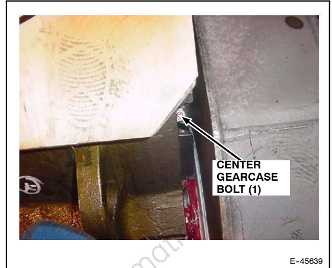
Figure 4. Motor Side (Center) Gearcase Split Line Bolt.
