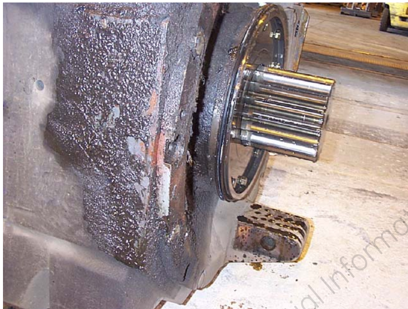
Figure 9. Typical Leaking Unit in Need of Service.
