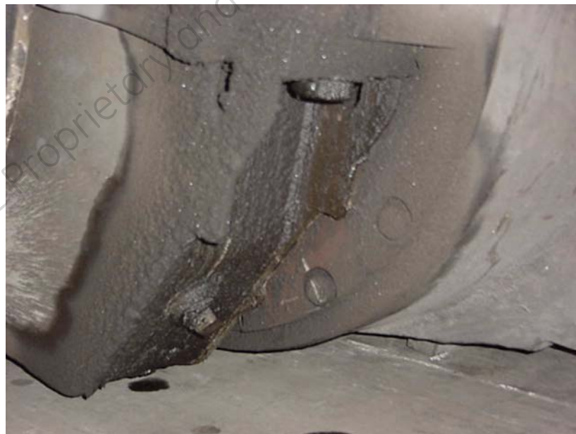
Figure 12. Typical Leaking Axle Bore Seals Or Split Line Leak.
