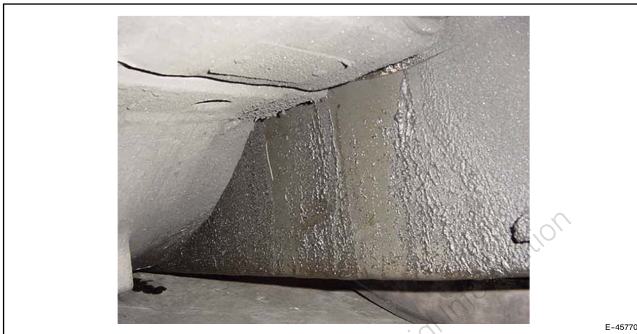
Figure 13. Typical Leaking Axle Bore Seal.
