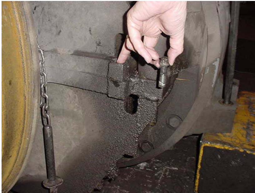
Figure 11. Typical Split Line Leak Due To Broken Bolt Or Missing Sealant.
