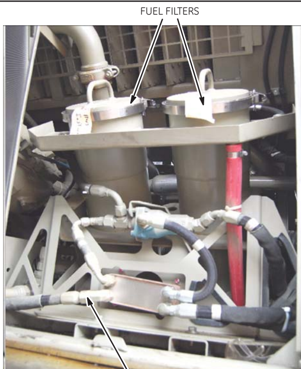
Figure 16. Fuel Filter Housing
