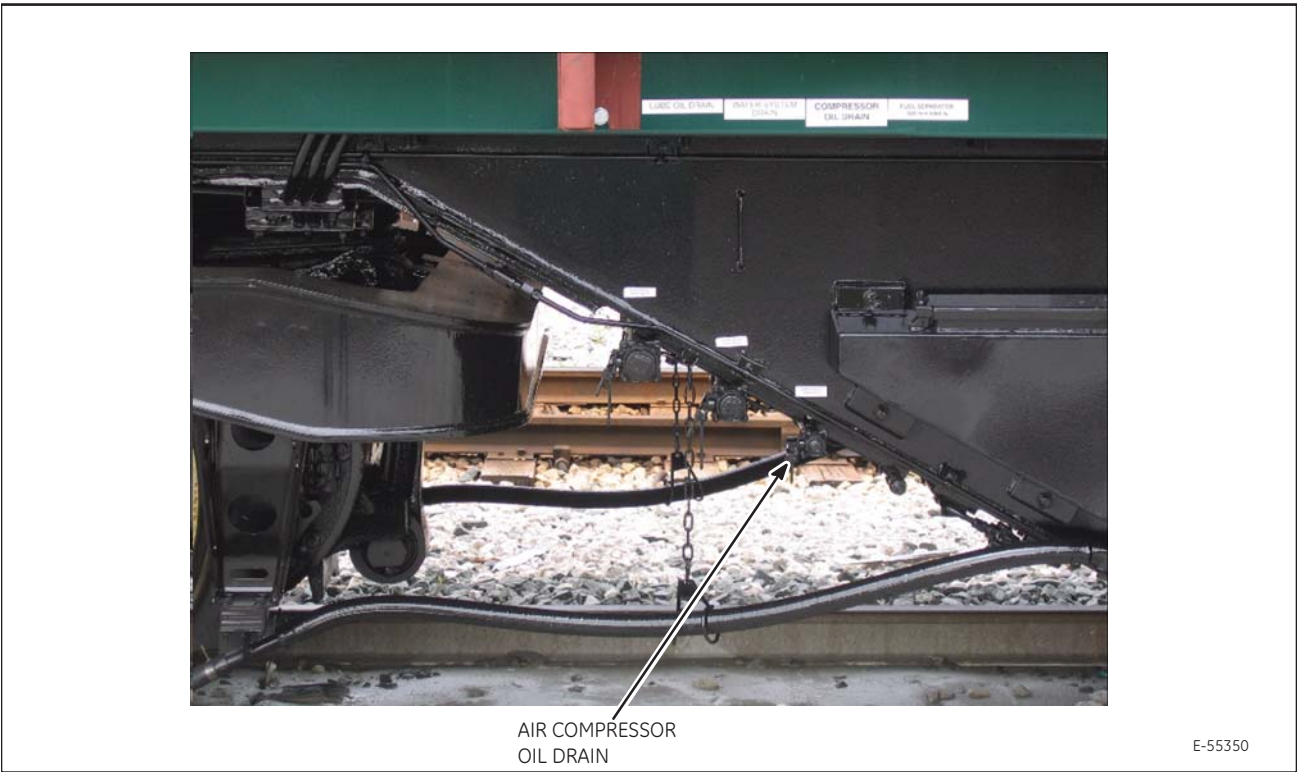
Figure 13. Air Compressor Oil Drain
