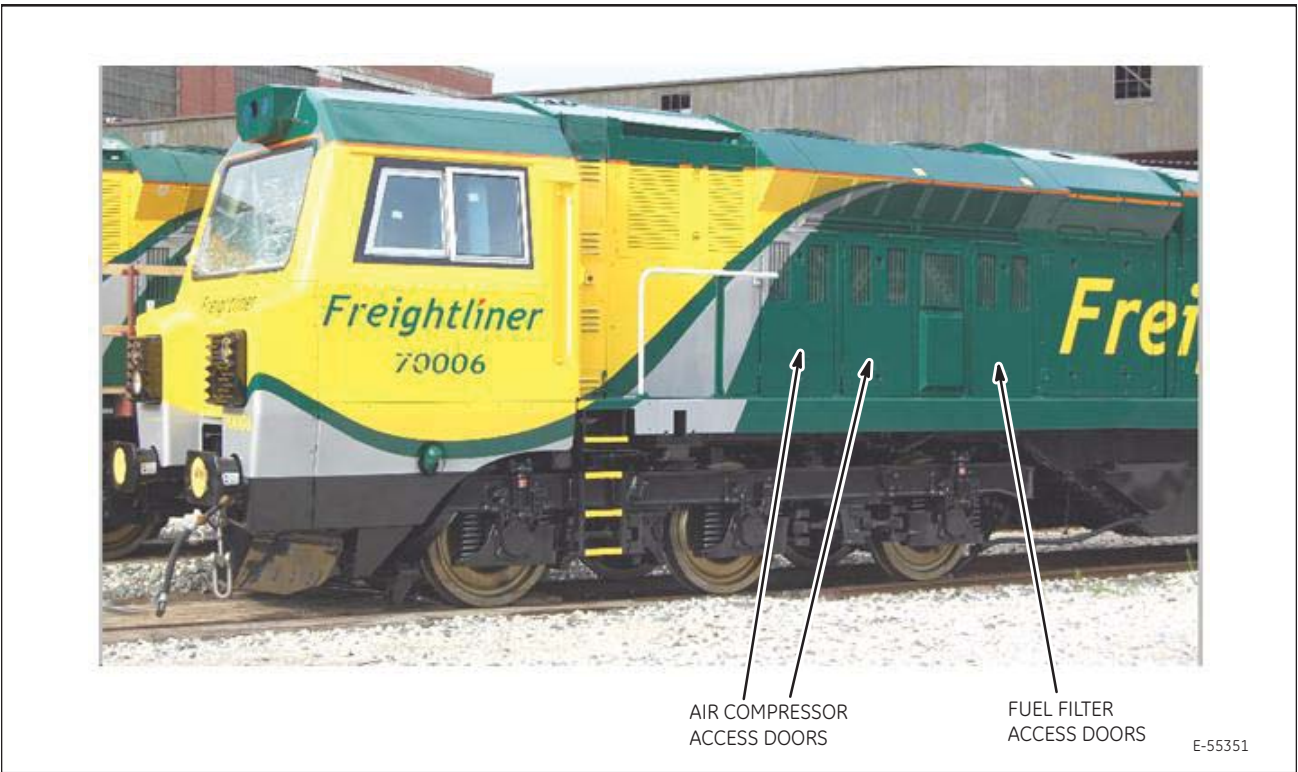
Figure 14. Air Compressor and Fuel Filter Access Doors
