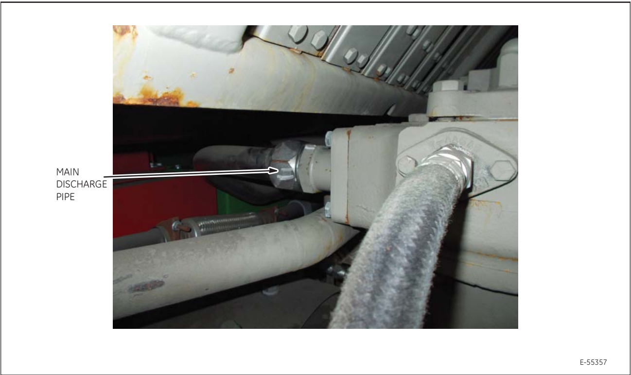
Figure 20. Main Discharge Pipe
